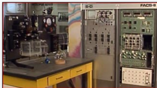
A FACS-II flow cytometer like the one that Don Mason installed.
