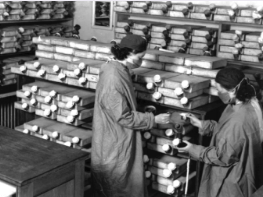
'Penicillin girls' tending the Heatley-designed vessels for growing penicillin mould at the Dunn School in 1939/40.
