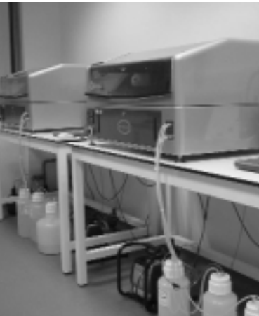
Contact microarray printers at the Dunn School have enabled population studies on the four key experimental strains of N.gonorrhoeae
