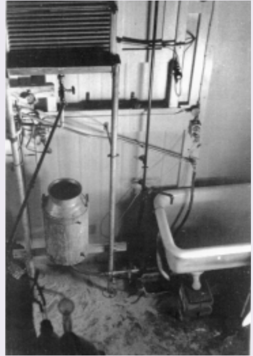
Above: Equipment used to extract penicillin at the Dunn School in 1939.
